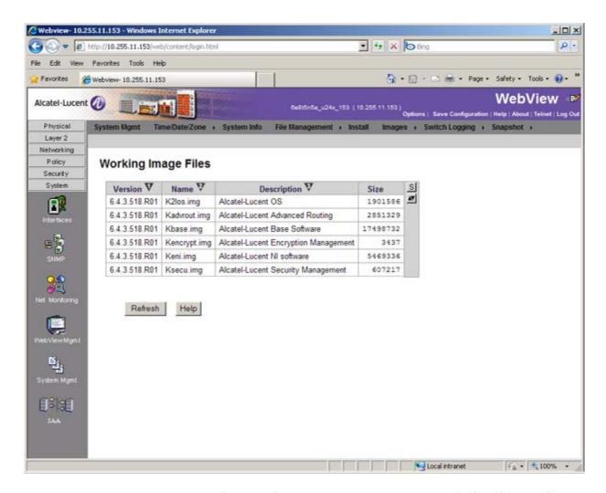
In addition, you should also select **System > System Mgmt > Images > Images in Certified** and **System > System Mgmt > Images > Images in Working** to verify that Certified and Working directories were successfully upgraded.
