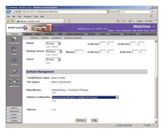
10 In the Software Management field, select Copy Working -> Certified on Primary for standalone switches. For a stack, select Copy Working -> Certified & Synchronize with Secondary and click Apply.
